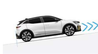
hill start assist. This system is enabled when the gradient is steeper than 3% by maintaining the brake pressure for two seconds.
