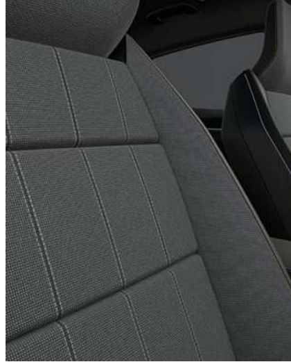
grey fabric made from recycled materials and black synthetic leather seat upholstery
